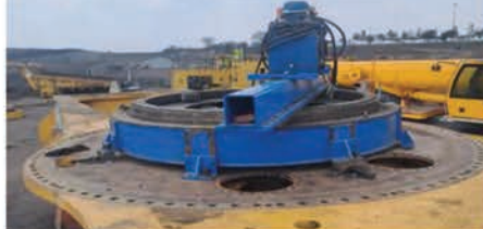
Slew bearing seat area - excavator
