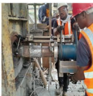
Paste Mixer shaft repairs
