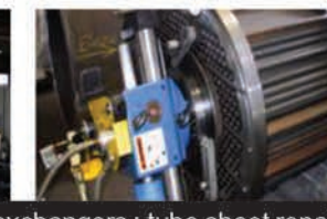
Facing of heat exchangers ; tube sheet repairs and replacement
