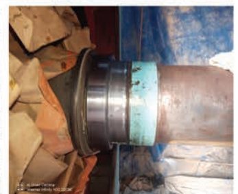
Facing of heat exchangers ; tube sheet repairs and replacement
