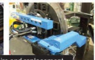
Facing of heat exchangers ; tube sheet repairs and replacement
