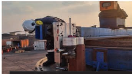
Slew bearing seat area - excavator
