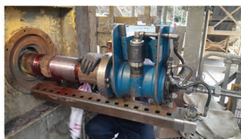
Facing of heat exchangers ; tube sheet repairs and replacement
